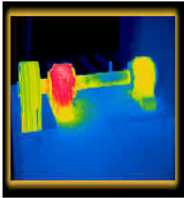
Figure E-5: Infrared image of an overheated bearing
