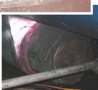
Crack with red dye penetrant
