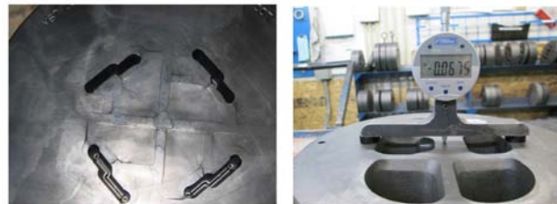
Figure 10-10: Cold Dies may result in broken die and/or wasted billets
