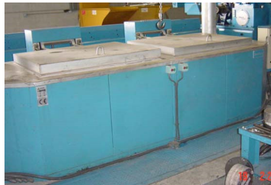
Figure 10-1: Box-type die heaters (Photo courtesy of Gia)
