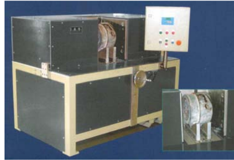
Figure 10-6: Induction die heater (Photo courtesy of IAS GmbH)
