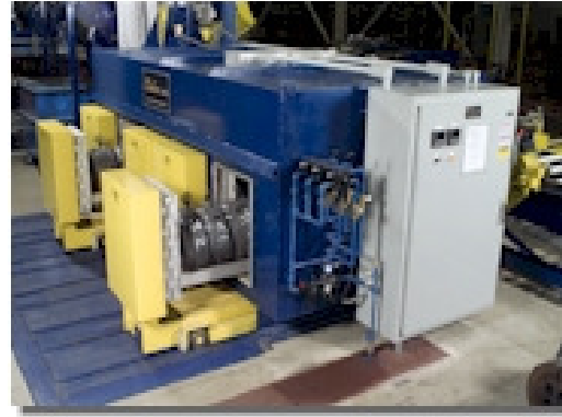
Figure 10-3: Drawer-type die heater (Photo courtesy of Belco Industries)
