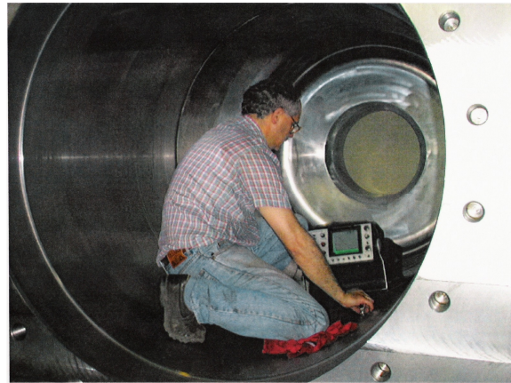
Figure 1-1: Ultrasound test of main cylinder (Photo courtesy of Presezi Extrusion)
