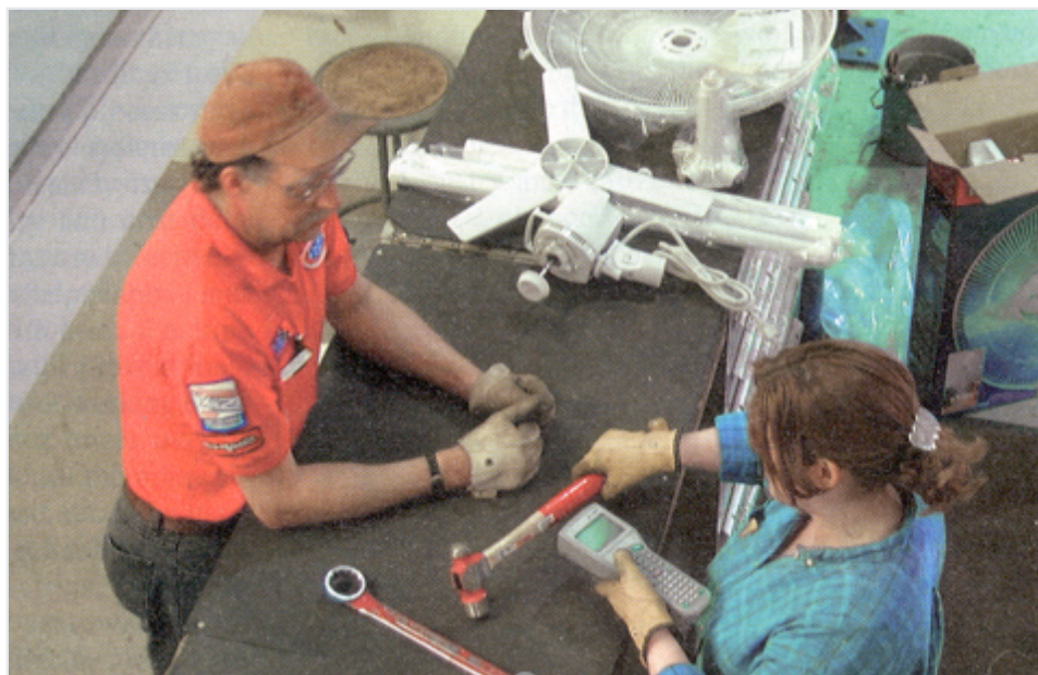
Figure E-11: Barcode identification and tracking of tools
