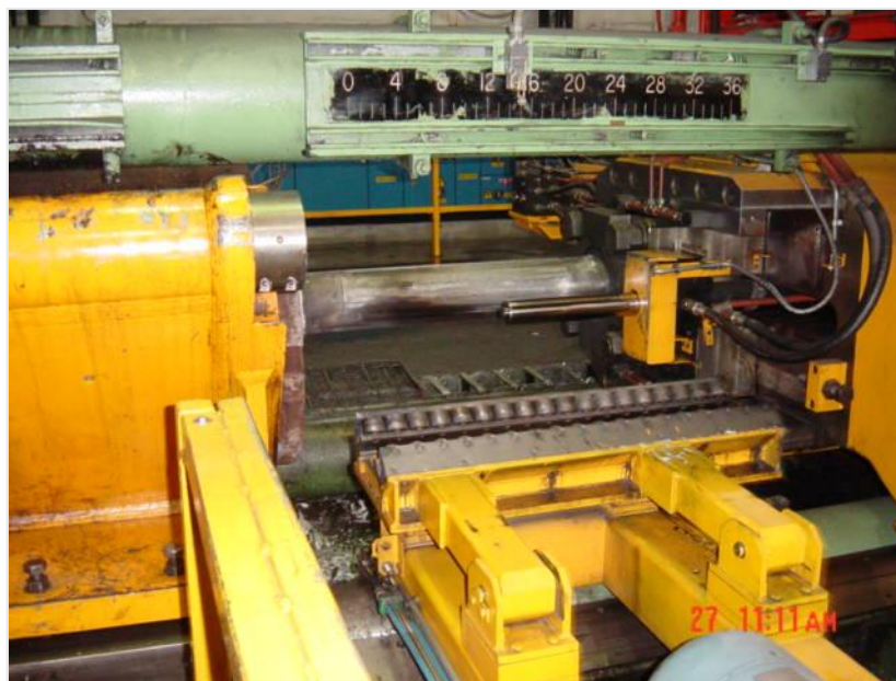
Figure C-10: Moveable stem conversion, showing horizontally-moving stem, billet pusher, and robot loader. Photo courtesy of OMAV
