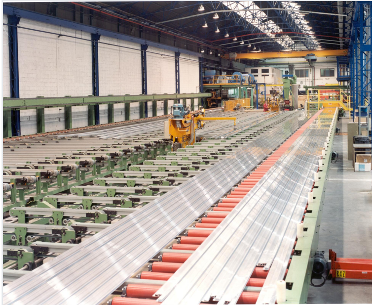
Figure C-24: Belt-type cooling table with saw feed conveyor (Photo courtesy of OMAV)
