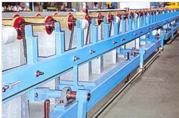
Figure C-21: Roller-type run-out table with cooling air ducts beneath (Photo courtesy of OMAV)
