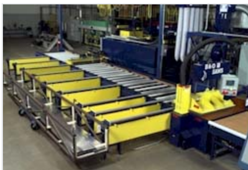
Figure C-26: Saw and length gauge-table with manual off-load belts (Photo courtesy of Belco)
