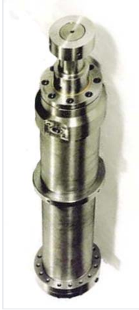
Figure B-4: Side or crosshead cylinders. After inspection, store in a vertical position to avoid any load on packing, and coat the inside and machined surfaces with oil. (Photo courtesy of Lake Park Tool)
