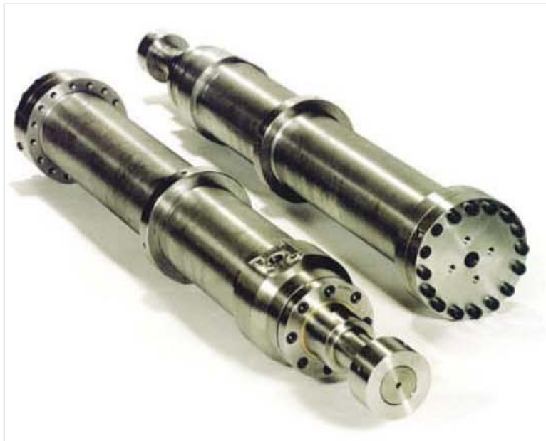
Figure B-4: Side or crosshead cylinders. After inspection, store in a vertical position to avoid any load on packing, and coat the inside and machined surfaces with oil. (Photo courtesy of Lake Park Tool)
