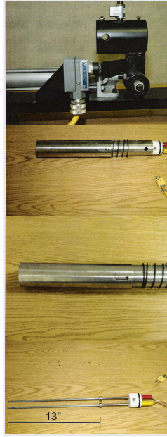
Figure 7-8: Disassembled components of thermocouple probe assembly (Photos courtesy of Belco)
