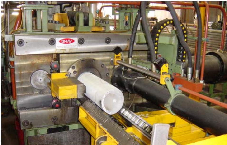
Figure 7-18: Horizontal-stroke log shear (Photo courtesy of OMAV)
