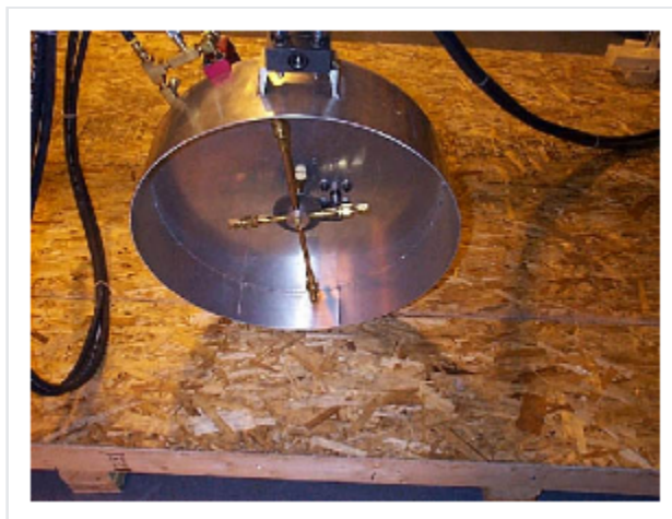
Figure 7-24: Spinning nozzle lubricant applicator for dummy block (Photo courtesy of Amcol)
