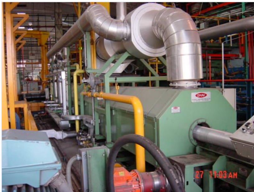
Figure 7-5: Gas-fired log heater with combustion air preheat (Photo courtesy of OMAV)
