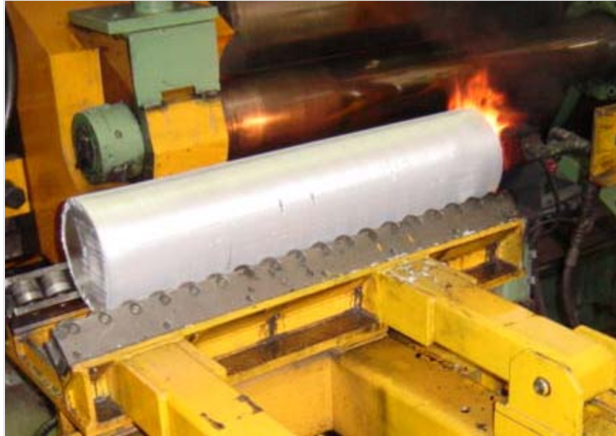
Figure 7-23: "Sooter" or flame lubricator for billet end (Photo courtesy of OMAV)
