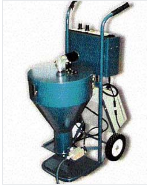
Figure 7-25: Applicator system for Boron Nitride powder (Photo courtesy of Castool)
