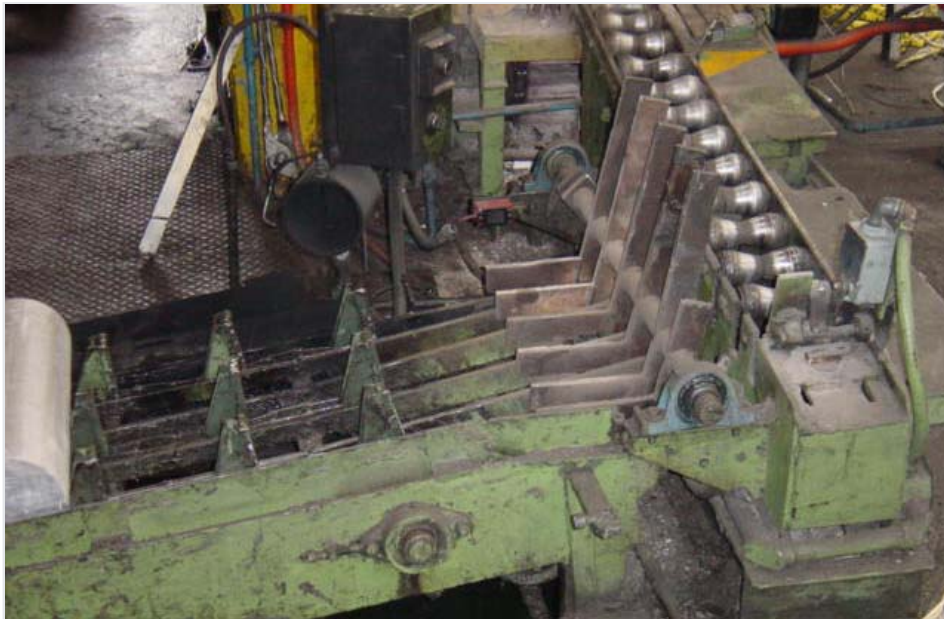
Figure 7-22: Pivot-arm billet transfer
