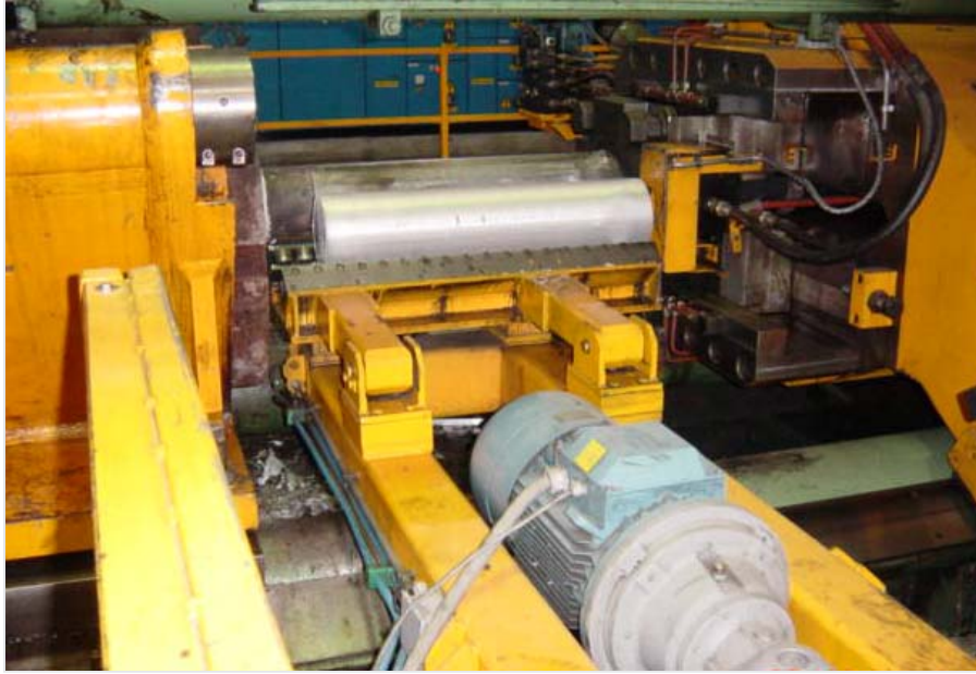
Figure 7-21: Robot-type billet transfer & loader (Photo courtesy of OMAV)
