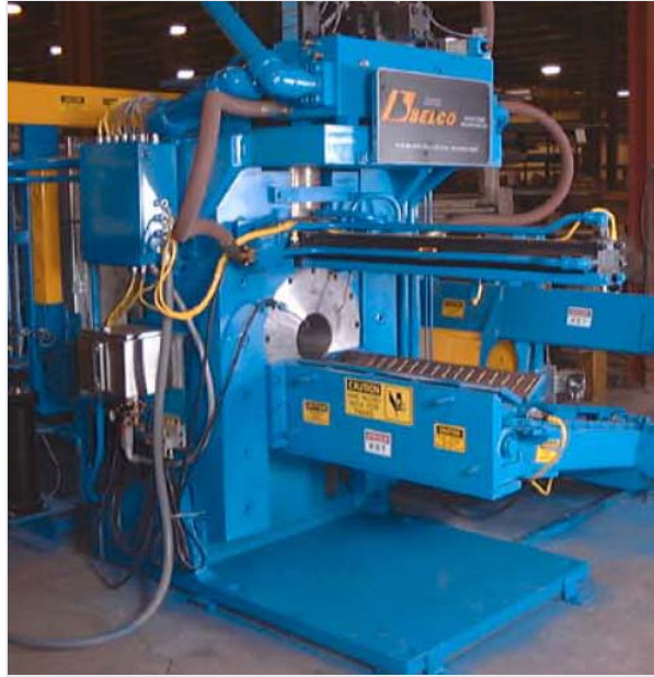
Figure 7-16: Vertical-stroke log shear (Photo courtesy of Belco)
