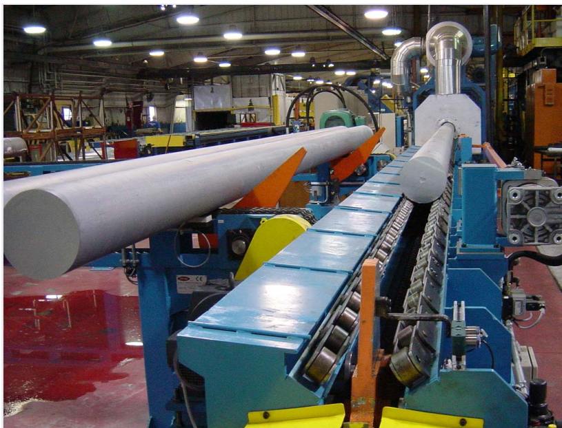
Figure 7-1: Log feed table and conveyor (Photo courtesy of OMAV)
