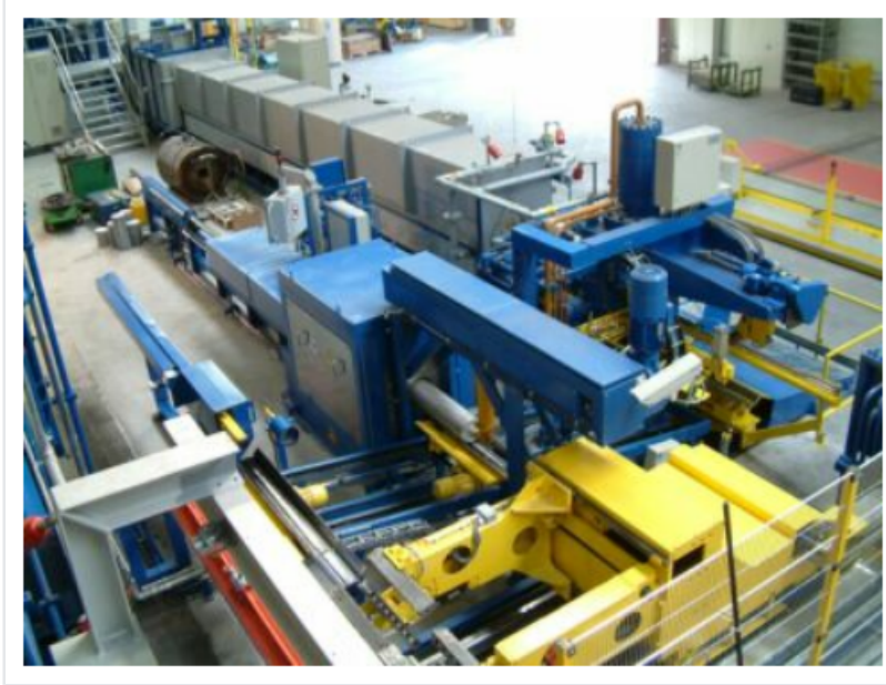
Figure 7-4: Gas-plus-induction billet heater (Photo courtesy of IAS)
