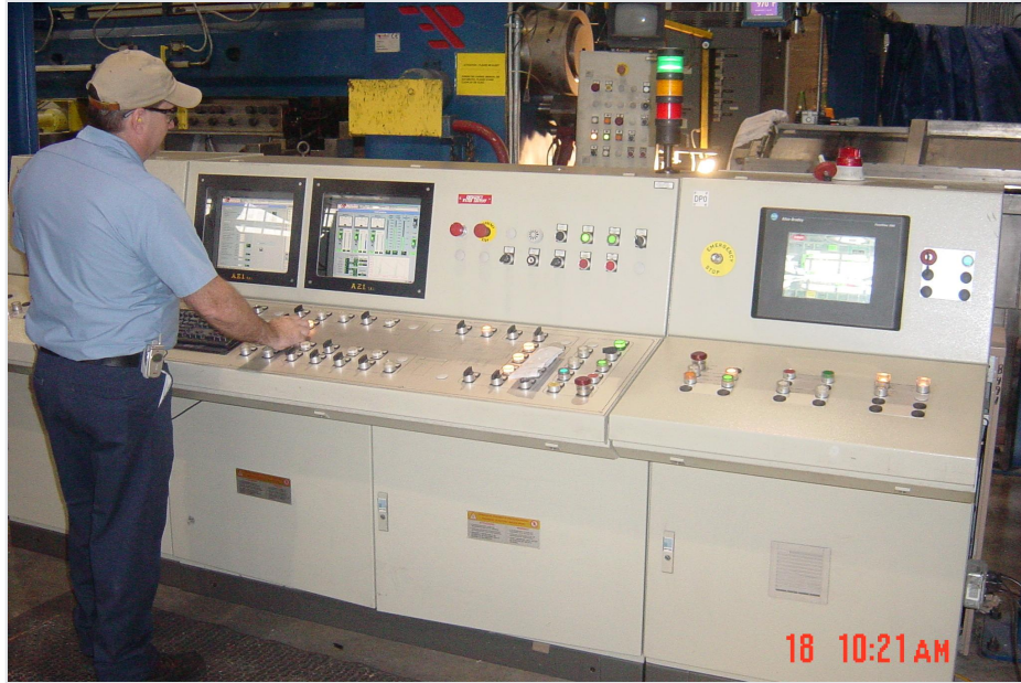
Figure 6-2: Modern control desk for entire press line with graphic operator interface (Photo courtesy of Presezzi Extrusion)
