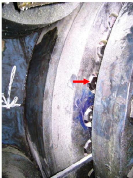
Figures 16a). A through-wall flange crack is mapped on the front face of the main cylinder flange. The gland packing ring had been removed to provide access for a UT straight beam examination. The crack was repaired, and the main cylinder was returned to service.
