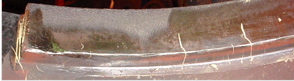
Magnetic particle shows cracks in a hot container housing
