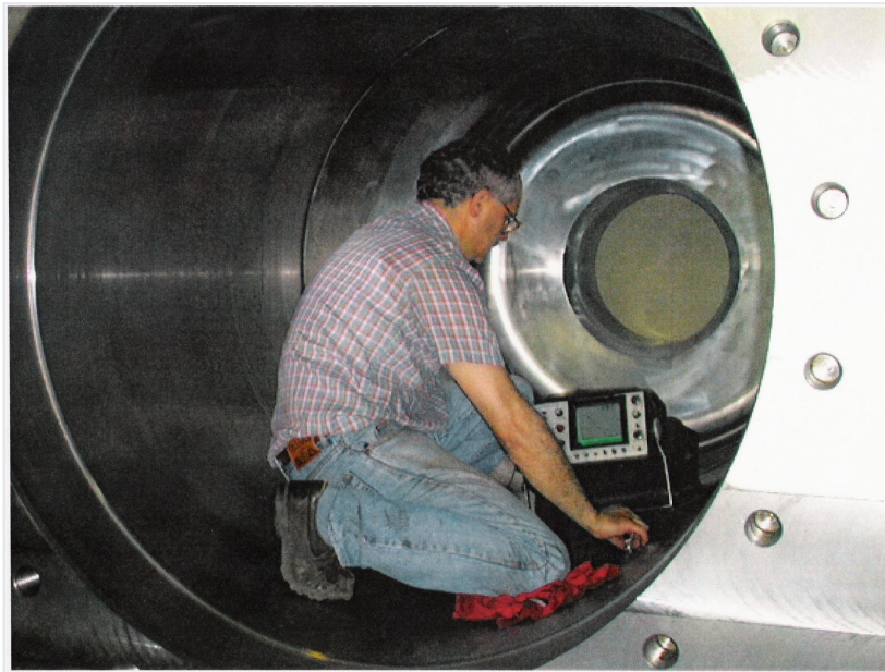
Figure 4-9: Ultrasound Test of Main Cylinder
