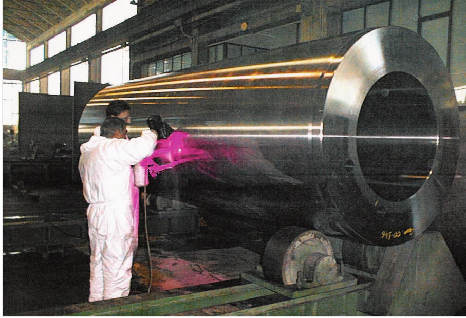
Figure 4-10: Magnetic Particle Test of Main Ram
