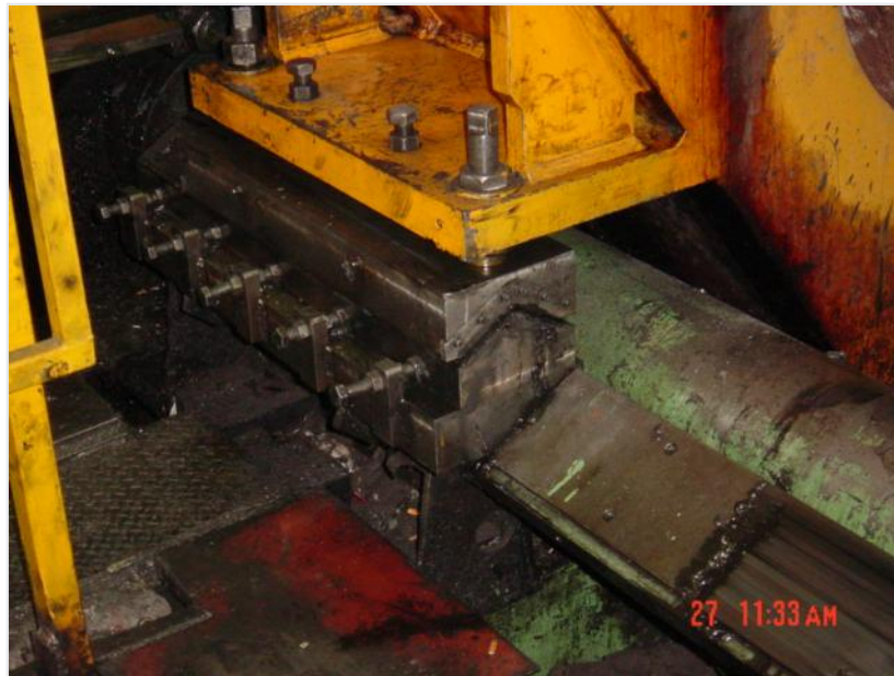
Figure 2-17: Container guides modified to V-type
