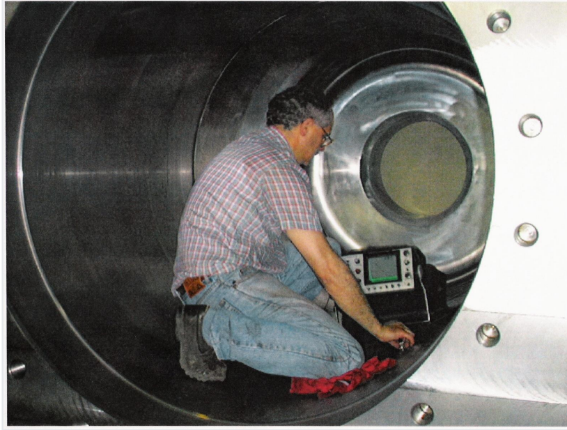
Figure 1-1: Ultrasound test of main cylinder (Photo courtesy of Presezzi Extrusion)
