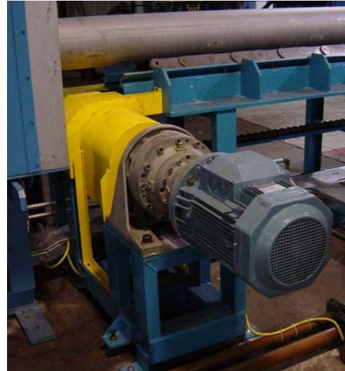
Figure 7-2: Log feed conveyor gear drive (Photo courtesy of OMAV)
