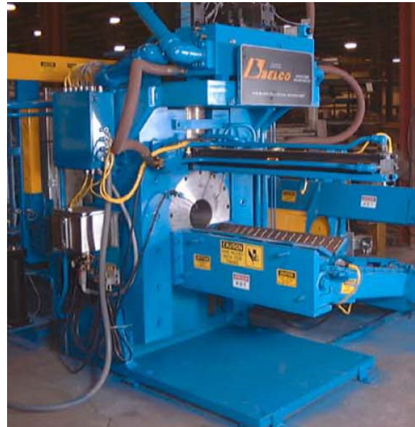
Figure 7-16: Vertical-stroke log shear (Photo courtesy of Belco)
