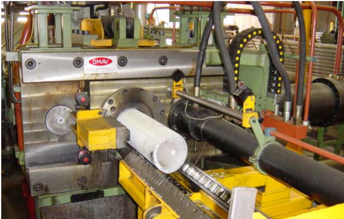
Figure 7-18: Horizontal-stroke log shear (Photo courtesy of OMAV)
