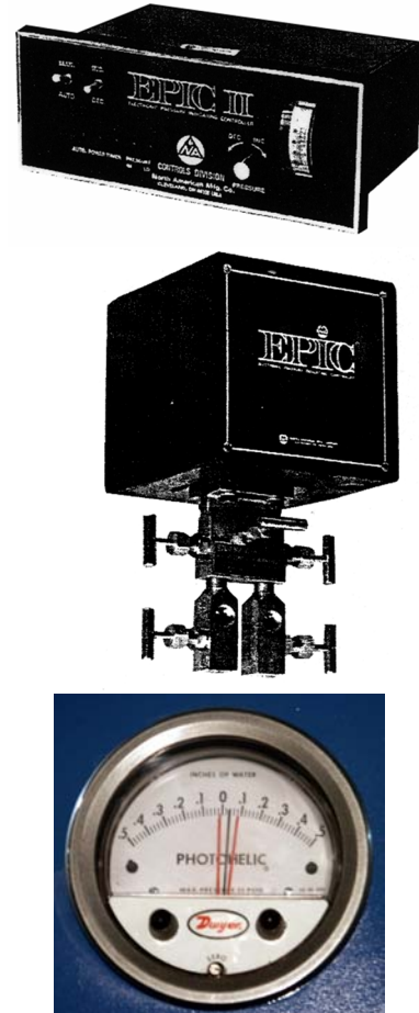
Figure 7-15: EPIC and Photohelic furnace pressure controllers
