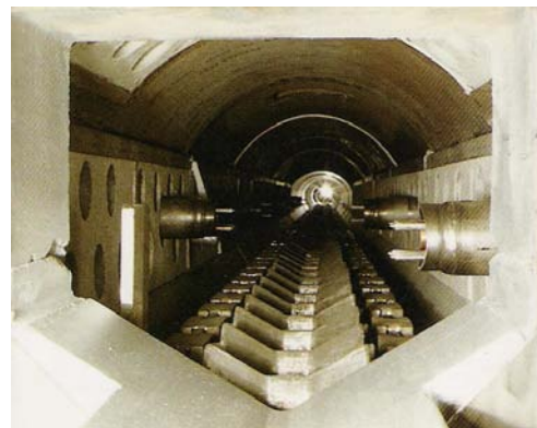
Figure 7-3: Cast alloy support rollers (Photo courtesy of OMAV)
