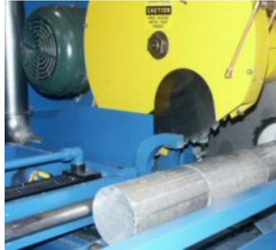
Figure 7-19: Hot log saw (Photo courtesy of Belco)
