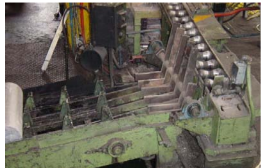
Figure 7-22: Pivot-arm billet transfer
