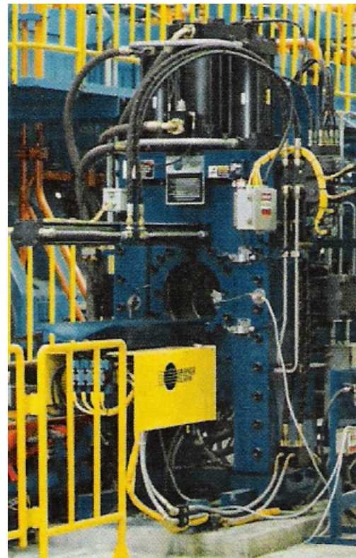
Figure 7-17: Vertical-stroke log shear (Photo courtesy of Granco Clark)
