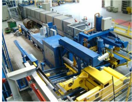
Figure 7-4: Gas-plus-induction billet heater (Photo courtesy of IAS)
