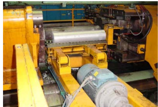
Figure 7-21: Robot-type billet transfer & loader (Photo courtesy of OMAV)
